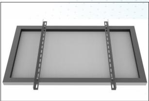
2. Fix the L feet to the brackets with M8 screws.
