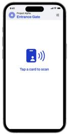
When tapping an NFC badge the person's profile card will automatically display with their permission to the selected zone. Granted workers are automatically checked-in or out when a fixed direction is set. Denied workers will require a manual tap by the app user to record the IN or OUT attempt.
